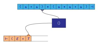
$$(E+\underline{T})*(a*a+a)\dashv \Rightarrow (E+\underline{F})*(a*a+a)\dashv \Rightarrow (\underline{E}+a)*(a*a+a)\dashv \Rightarrow \dots$$
