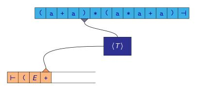
$$(E+\underline{T})*(a*a+a)\dashv \Rightarrow (E+\underline{F})*(a*a+a)\dashv \Rightarrow (\underline{E}+a)*(a*a+a)\dashv \Rightarrow \dots$$
