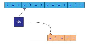
$$\cdots \Rightarrow (\underline{F} + T) * F \dashv \Rightarrow (a + \underline{T}) * F \dashv \Rightarrow (a + \underline{F}) * F \dashv \Rightarrow (a + a) * \underline{F} \dashv$$
