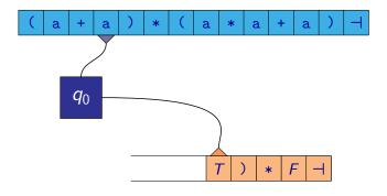
$$\cdots \ \Rightarrow \ (\underline{F} + T) * F \dashv \ \Rightarrow \ (\underline{T} + T) * F \dashv \ \Rightarrow \ (\underline{F} + T) * F \dashv \ \Rightarrow \ (\underline{a} + \underline{T}) * F \dashv$$
