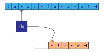
$$\cdots \ \Rightarrow \ (\underline{F} + T) * F \dashv \ \Rightarrow \ (\underline{T} + T) * F \dashv \ \Rightarrow \ (\underline{F} + T) * F \dashv \ \Rightarrow \ (\underline{a} + \underline{T}) * F \dashv$$
