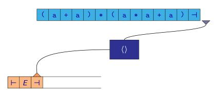
$$\underline{E} \dashv \ \Rightarrow \ \underline{T} \dashv \ \Rightarrow \ T * \underline{F} \dashv \ \Rightarrow \ T * (\underline{E}) \dashv \ \Rightarrow \ T * (E + \underline{T}) \dashv \ \Rightarrow \ \cdots$$
