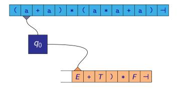
$$\cdots \ \Rightarrow \ \underline{T} \dashv \ \Rightarrow \ \underline{T} * F \dashv \ \Rightarrow \ \underline{F} * F \dashv \ \Rightarrow \ (\underline{E}) * F \dashv \ \Rightarrow \ (\underline{E} + T) * F \dashv$$
