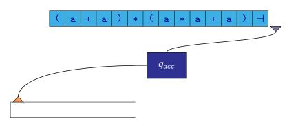
$$\underline{S} \ \Rightarrow \ \underline{E} \ \dashv \ \Rightarrow \ \underline{T} \ \dashv \ \Rightarrow \ T * \underline{F} \ \dashv \ \Rightarrow \ T * (\underline{E}) \ \dashv \ \Rightarrow \ T * (E + \underline{T}) \ \dashv \ \Rightarrow \ \cdots$$
