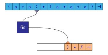
$$\cdots \Rightarrow (\underline{F} + T) * F \dashv \Rightarrow (a + \underline{T}) * F \dashv \Rightarrow (a + \underline{F}) * F \dashv \Rightarrow (a + a) * \underline{F} \dashv$$
