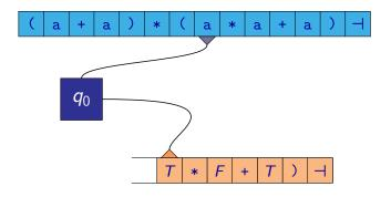
$$\cdots \Rightarrow (a+a)*(\underline{E}+T)\dashv \Rightarrow (a+a)*(\underline{T}+T)\dashv \Rightarrow (a+a)*(\underline{T}*F+T)\dashv$$
