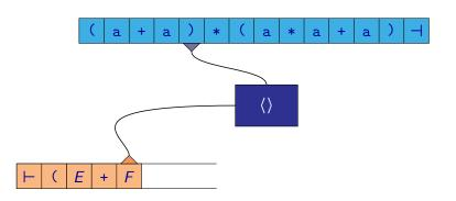
$$(\underline{E}+\underline{F})*(a*a+a)\dashv \Rightarrow (\underline{E}+a)*(a*a+a)\dashv \Rightarrow (\underline{T}+a)*(a*a+a)\dashv \Rightarrow \dots$$
