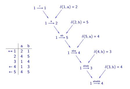
A word  $w \in \Sigma^*$  is **accepted** by a deterministic finite automaton  $\mathcal{A} = (Q, \Sigma, \delta, q_0, F)$  iff there exists a state  $q \in F$  such that  $q_0 \xrightarrow{w} q$ .
