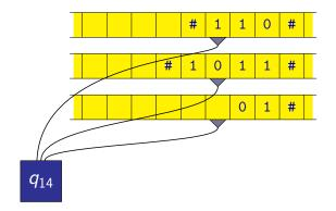
Multitape machines often use one of its tapes as an input tape and one of its tapes as an output tape. Other tapes are used as working tapes:
