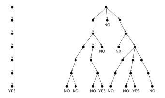
A nondeterministic finite automaton accepts a given word if there **exists** at least one computation of the automaton that accepts the word.
