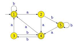
A **deterministic finite automaton** consists of **states** and **transitions**. One of the states is denoted as an **initial state** and some of states are denoted as **accepting**. Formally, a deterministic finite automaton (DFA) is defined as a tuple
