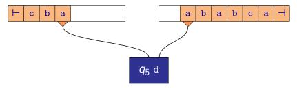
A tape, infinite on both sides, can be simulated by two stacks:
